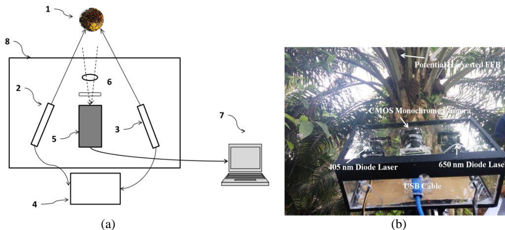
Figure 2. LIFI System (a) system schematic, (b) system on tripod 2 m from a 3 m height of an oil palm tree
